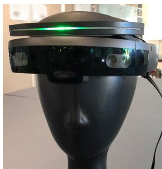
Figure 2: Modified HoloLens device with external LED display.
