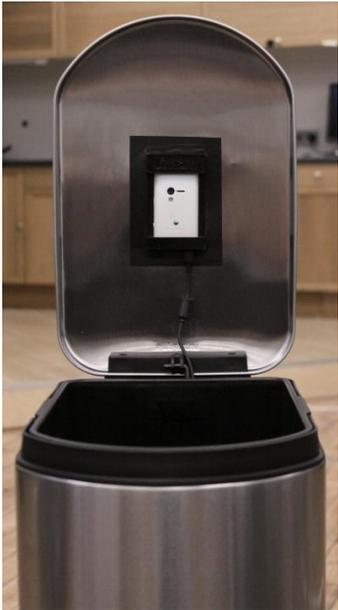
**Figure 1:** Kitchen bin augmented with Internet-enabled mobile phone (Sony Ericsson Xperia X10 mini).
