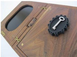
**Figure 2:** Opened box artifact with a screen to the left and a key object (including the RFID tag) to the right.
