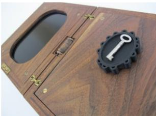
**Figure 2:** Opened box artifact with a screen to the left and a RFID tag containing object to the right to trigger the display of a video message.
